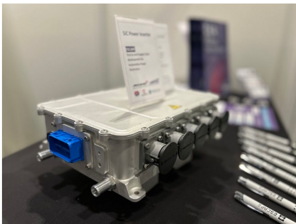
Prototype of McLaren Applied's 800V SiC Inverter
